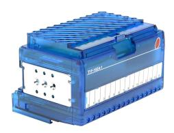
Terminator analog output module, 16-channel, current, 12-bit, external 24 VDC required. Requires T1K-16B or T1K-16B-1 terminal base.
