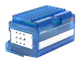
Terminator analog output module, 16-channel, current, 12-bit, output current signal range(s) of 0-20 mA and 4-20 mA, external 24 VDC required.
