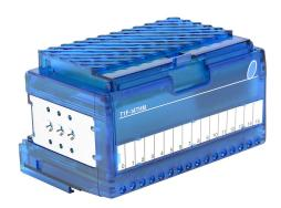
Terminator temperature input module, thermocouple, 14-channel, 12-bit resolution, input thermocouple type(s): J, E, K, R, S, T, B, N, C. Requires T1K-16B or T1K-16B-1 terminal base.
