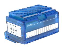
Terminator temperature input module, thermocouple, 14-channel, 12-bit resolution, input thermocouple type(s): J, E, K, R, S, T, B, N, C. Requires T1K-16B or T1K-16B-1 terminal base.
