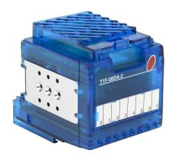
Terminator analog output module, 8-channel, voltage, 12-bit, output voltage signal range(s) of 0-5 VDC, 0-10 VDC, +/- 5 VDC and +/- 10 VDC, external 24 VDC required.
