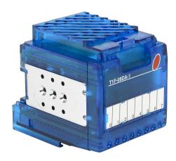
Terminator analog output module, 8-channel, current, 12-bit, output current signal range(s) of 0-20 mA and 4-20 mA, external 24 VDC required.
