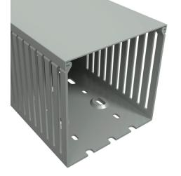
Iboco T1E series open slot narrow finger wire duct, 4in width, 4in height, 3.2ft/1m length, gray. Cover included.
