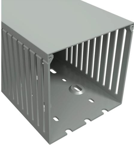
Iboco T1E series open slot narrow finger wire duct, 4in width, 4in height, 3.2ft/1m length, gray. Cover included.
