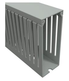
Iboco T1E series open slot narrow finger wire duct, 1.5in width, 4in height, 6.5ft/2m length, gray. Cover included.
