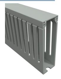
Iboco T1E series open slot narrow finger wire duct, 1in width, 3in height, 3.2ft/1m length, gray. Cover included.
