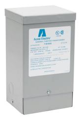
ACME buck-boost transformer, encapsulated core, 750 VA, 1-phase, 120/240 VAC primary, 16/32 VAC secondary, 50/60 Hz, NEMA 3R, wall mount.
