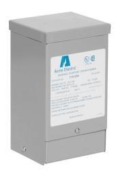
ACME buck-boost transformer, encapsulated core, 500 VA, 1-phase, 120/240 VAC primary, 16/32 VAC secondary, 50/60 Hz, NEMA 3R, wall mount.
