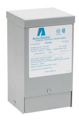
ACME buck-boost transformer, encapsulated core, 500 VA, 1-phase, 120/240 VAC primary, 12/24 VAC secondary, 50/60 Hz, NEMA 3R, wall mount.
