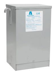
ACME buck-boost transformer, encapsulated core, 5 kVA, 1-phase, 240/480 VAC primary, 24/48 VAC secondary, 60 Hz, NEMA 3R, wall mount.
