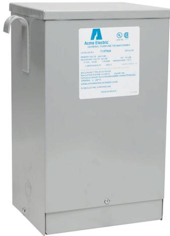
ACME buck-boost transformer, encapsulated core, 5 kVA, 1-phase, 240/480 VAC primary, 24/48 VAC secondary, 60 Hz, NEMA 3R, wall mount.
