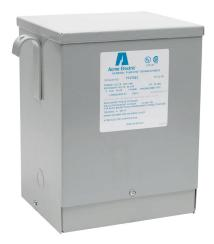
ACME buck-boost transformer, encapsulated core, 3 kVA, 1-phase, 240/480 VAC primary, 24/48 VAC secondary, 60 Hz, NEMA 3R, wall mount.
