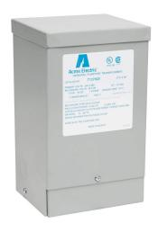
ACME buck-boost transformer, encapsulated core, 1 kVA, 1-phase, 240/480 VAC primary, 24/48 VAC secondary, 60 Hz, NEMA 3R, wall mount.
