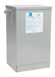
ACME buck-boost transformer, encapsulated core, 5 kVA, 1-phase, 120/240 VAC primary, 16/32 VAC secondary, 60 Hz, NEMA 3R, wall mount.
