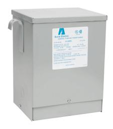
ACME buck-boost transformer, encapsulated core, 3 kVA, 1-phase, 120/240 VAC primary, 16/32 VAC secondary, 60 Hz, NEMA 3R, wall mount.
