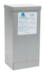
ACME buck-boost transformer, encapsulated core, 2 kVA, 1-phase, 120/240 VAC primary, 16/32 VAC secondary, 60 Hz, NEMA 3R, wall mount.
