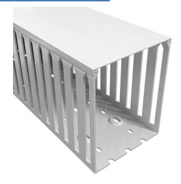
Iboco T1 series open slot wide finger wire duct, 4in width, 5in height, 6.5ft/2m length, white. Cover included.
