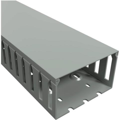
lboco T1 series open slot wide finger wire duct, 4in width, 2.25in height, 6.5ft/2m length, gray. Cover included.
