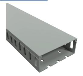
Iboco T1 series open slot wide finger wire duct, 4in width, 1.5in height, 6.5ft/2m length, gray. Cover included.
