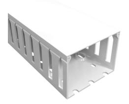
Iboco T1 series open slot wide finger wire duct, 3in width, 2.25in height, 6.5ft/2m length, white. Cover included.
