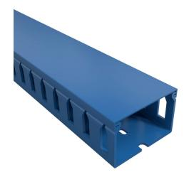
Iboco T1 series open slot wide finger wire duct, 2.25in width, 1.5in height, 6.5ft/2m length, blue. Cover included.
