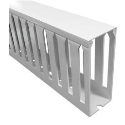
Iboco T1 series open slot wide finger wire duct, 1.5in width, 4in height, 6.5ft/2m length, white. Cover included.
