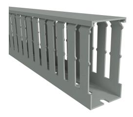
Iboco T1 series open slot wide finger wire duct, 1.5in width, 3in height, 3.2ft/1m length, gray. Cover included.
