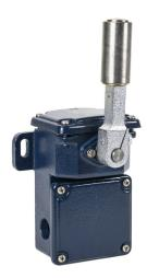
Schmersal heavy duty limit switch, side rotary lever with metal belt roller, (2) N.C. contact(s), slow action, 122mm hole spacing, cast iron, (2) M25 x 1.5 cable entry.
