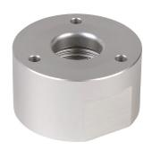
Patlite threaded pole adapter, 40mm diameter, 1/2in NPT thread, silver, aluminum. For use with Patlite LR4 series direct mount signal tower bases. (3) screw-tapped spacers included.
