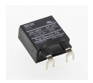
Fuji Electric surge suppressor, resistor-capacitor, 24-48 VAC/VDC. For use with SC-E02x, SC-E03x, SC-E04x and SC-E05x contactors.
