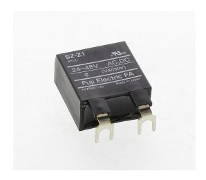
Fuji Electric surge suppressor, varistor, 24-48 VAC/VDC. For use with SC-E02x, SC-E03x, SC-E04x and SC-E05x contactors.
