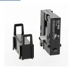
Fuji Electric mechanical interlock, for use with SC-E02x, SC-E03x, SC-E04x, SC-E05x, SC-E1x, SC-E2x, SC-E2Sx, SC-E3x and SC-E4x contactors, mechanically connects contactors to prevents both from being pulled in at the same time.
