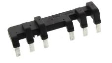
Fuji Electric reversing connection bar, line side only mount. For use with SC-E3x and SC-E4x contactors.
