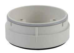
Patlite 4-hole adapter, top mount, 70mm diameter, 14mm height, off-white, ABS plastic. For use with LS7 series signal towers.
