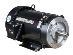
Marathon Symax super premium efficiency AC permanent magnet motor, high-performance inverter duty, 10hp, 3-phase, 230/460 VAC, 1800rpm, TEFC, 215TC frame, rolled steel, C-face/rigid base mount. Requires drive.
