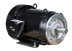
Marathon Symax super premium efficiency AC permanent magnet motor, high-performance inverter duty, 7-1/2hp, 3-phase, 230/460 VAC, 1800rpm, TEFC, NEMA 213TC frame, rolled steel, C-face/rigid base mount. Requires drive.
