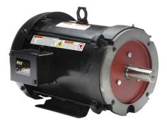
Marathon Symax super premium efficiency AC permanent magnet motor, high-performance inverter duty, 5hp, 3-phase, 230/460 VAC, 1800rpm, TEFC, NEMA 184TC frame, rolled steel, Cface/rigid base mount. Requires drive.
