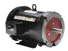
Marathon Symax super premium efficiency AC permanent magnet motor, high-performance inverter duty, 5hp, 3-phase, 230/460 VAC, 1800rpm, TEFC, 184TC frame, rolled steel, C-face/rigid base mount. Requires drive.
