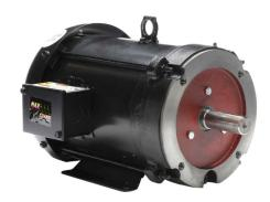
Marathon Symax super premium efficiency AC permanent magnet motor, high-performance inverter duty, 3hp, 3-phase, 230/460 VAC, 1800rpm, TEFC, NEMA 182TC frame, rolled steel, C-face/rigid base mount. Requires drive.
