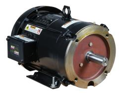
Marathon Symax super premium efficiency AC permanent magnet motor, high-performance inverter duty, 3hp, 3-phase, 230/460 VAC, 1200rpm, TEFC, NEMA 182TC frame, rolled steel, Cface/rigid base mount. Requires drive.
