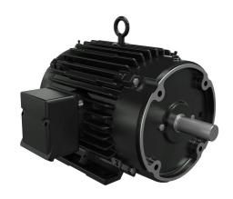
Marathon Symax super premium efficiency AC permanent magnet motor, high-performance inverter duty, 5hp, 3-phase, 230/460 VAC, 1800rpm, TENV, 184TC frame, cast iron, C-face/rigid base mount. Requires drive.
