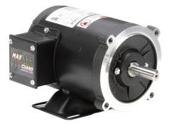
Marathon Symax premium efficiency AC permanent magnet motor, high-performance inverter duty, 1-1/2hp, 3-phase, 230/460 VAC, 1800rpm, TENV, NEMA S56C frame, rolled steel, Cface/rigid base mount. Requires drive.
