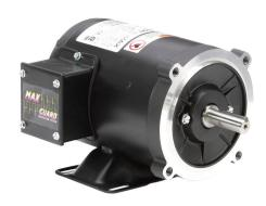
Marathon Symax premium efficiency AC permanent magnet motor, high-performance inverter duty, 1-1/2hp, 3-phase, 230/460 VAC, 1800rpm, TENV, S56C frame, rolled steel, C-face/rigid base mount. Requires drive.
