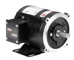
Marathon Symax premium efficiency AC permanent magnet motor, high-performance inverter duty, 1hp, 3-phase, 230/460 VAC, 1800rpm, TENV, S56C frame, rolled steel, C-face/rigid base mount. Requires drive.
