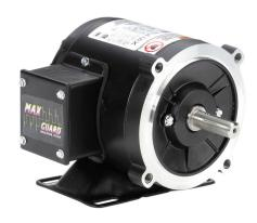
Marathon Symax premium efficiency AC permanent magnet motor, high-performance inverter duty, 1/2hp, 3-phase, 230/460 VAC, 1800rpm, TENV, NEMA S56C frame, rolled steel, C-face/rigid base mount. Requires drive.
