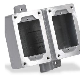
Killark device/splice box, dead end, (2) gang, (1) 3/4in female NPT conduit entries, aluminum. Use with XCS series cover assemblies for hazardous locations.
