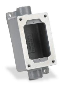
Killark device/splice box, feed through, (1) gang, (2) 3/4in female NPT conduit entries, aluminum. Use with XCS series cover assemblies for hazardous locations.
