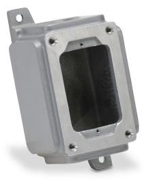
Killark device/splice box, deep dead end, (1) gang, (1) 3/4in female NPT conduit entries, aluminum. Use with XCS series cover assemblies for hazardous locations.
