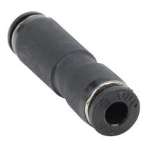
NITRA pneumatic push-to-connect fitting, union straight stop valve, thermoplastic (PBT) body, (1) 5/32in (4mm) push-to-connect to (1) 5/32in (4mm) push-to-connect. Package of 5.
