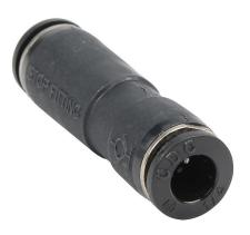
NITRA pneumatic push-to-connect fitting, union straight stop valve, thermoplastic (PBT) body, (1) 1/4in push-to-connect to (1) 1/4in push-to-connect. Package of 5.
