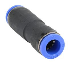
NITRA pneumatic push-to-connect fitting, union straight stop valve, thermoplastic (PBT) body, (1) 10mm push-to-connect to (1) 10mm push-to-connect. Package of 5.
