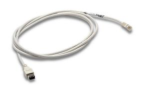
ZIPLink servo cable, 6-pin RJ12 to 6-pin IEEE connector, shielded, twisted pair, RS-485, 6.5ft/2m cable length. For use with SureServo amplifiers.
