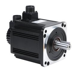
SureServo2 low inertia AC brushless servo motor, 2 kW, 3-phase input, 24-bit (16777216 ppr) encoder. For use with SureServo2 SV2A-4200 2 kW drive.
