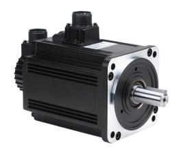
SureServo2 low inertia AC brushless servo motor, 2 kW, 3-phase input, 24-bit (16777216 ppr) encoder, integrated brake. For use with SureServo2 SV2A-4200 2 kW drive.
