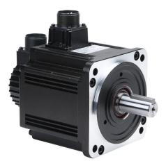
SureServo2 low inertia AC brushless servo motor, 1.5 kW, 3-phase input, 24-bit (16777216 ppr) encoder. For use with SureServo2 SV2A-4150 1.5 kW drive.
