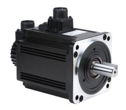
SureServo2 low inertia AC brushless servo motor, 1.5 kW, 3-phase input, 24-bit (16777216 ppr) encoder, integrated brake. For use with SureServo2 SV2A-4150 1.5 kW drive.
